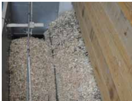
Flat store with a floor conveyor. Delivery occurs via rods, which either push or draw.
