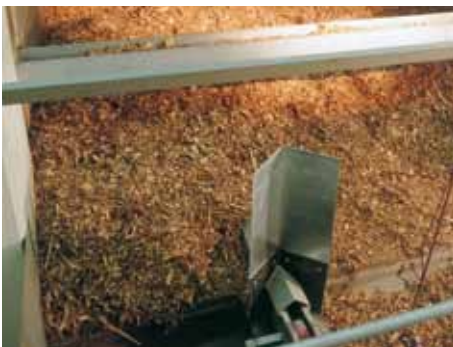
Flat store with a floor conveyor. Delivery occurs via rods, which either push or draw.
